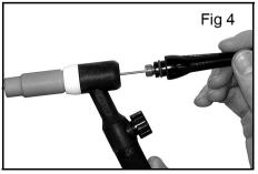
move, adjust it so that it protrudes from the nozzle by 4 - 5mm, and then tighten the end cap against the rubber O-ring. The electrode will now be secured in position.
